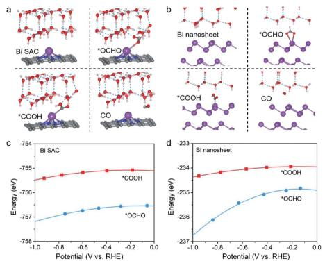
Fig. 1 Geometric structures of the 2e CO<sub>2</sub>RR species for (a) the Bi-N-C SAC and (b) the Bi nanosheets. The violet, grey, red, and white spheres denote Bi, C, O, and H, respectively. The blue dashed lines indicate the hydrogen bond. Computed total energies of \*OCHO and \*COOH on (c) the Bi-N-C SAC and (d) the Bi nanosheets as a function of potential.
