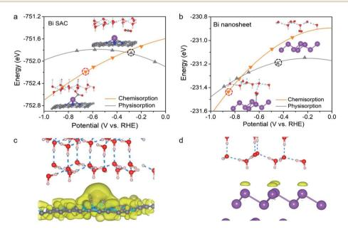
Fig. 2 Calculated total energies of chemisorbed  $CO_2$  (\* $CO_2$ ) and physisorbed  $CO_2$  of (a) the Bi-N-C SAC and (b) the Bi nanosheets as a function of potential U. Charge density difference for (c) the Bi-N-C SAC and (d) the Bi nanosheets when the applied potential changes from 0 to -0.6 V. The iso-value is 0.0006 a.u.
