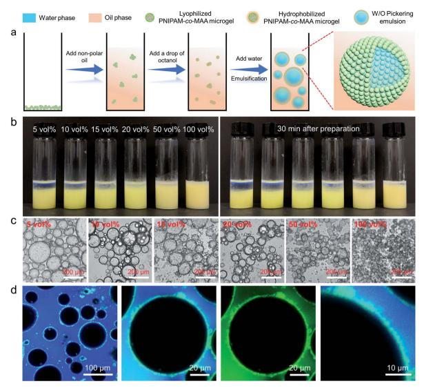
(a) Schematic illustration of the preparation process and stabilization mechanism of inverse W/O Pickering emulsions stabilized by octanol-swollen PNIPAM-co-MAA microgels. (b) Photographs and (c) optical microscopy images of inverse W/O Pickering emulsions (W: O = 1:1, v/v) stabilized by 1 wt% PNIPAM-co-MAA microgels in the oil phase and containing different concentrations of octanol. (d) CLSM images of the inverse W/O Pickering emulsion containing 20 vol% octanol.
