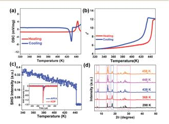
Fig. 2 Phase transition of APFA. (a) DSC curve. (b) Temperature-dependent  $\varepsilon'$  at 1 MHz. (c) Temperature-dependent SHG response. Inset: comparison of the SHG intensity of APFA and KDP. (d) Variable-temperature PXRD patterns.
