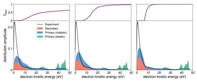
Fig. 7 Influence of  $f_{\rm elec}$ . Comparison of simulated spectra to experimental results for a photon energy corresponding to harmonic 37 of  $\approx$  800 nm ( $\approx$  57.6 eV), using several  $f_{\rm elec}$ . Left: amorphous ice. Middle: water vapour. Right: suggested sharper closing of electronic channels.
