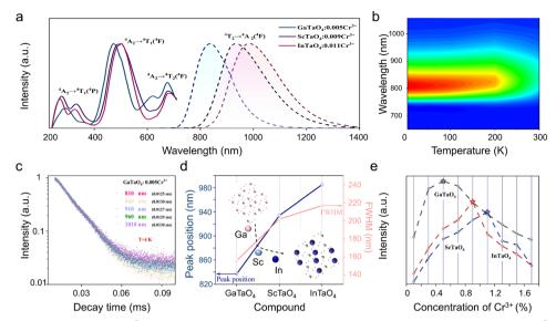
Fig. 2 (a) PLE and PL spectrum of  $XTaO_4$ : $Cr^{3+}$  (X = In, Sc, and Ga); (b) the low-temperature emission spectra of  $GaTaO_4$ : $Cr^{3+}$ ; (c) decay curves of  $GaTaO_4$ : $Cr^{3+}$  were monitored at 810 nm, 860 nm, 910 nm, 960 nm, and 1010 nm; (d) variation trend of the PL intensity of  $XTaO_4$ : $Cr^{3+}$  (X = In, Sc, and Ga) with  $Cr^{3+}$ -ion concentration; (e) the peaking position and FWHM of  $XTaO_4$ : $Cr^{3+}$  (X = In, Sc, and Ga).
