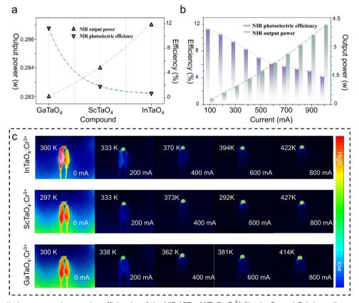
Fig. 4 (a) Output optical powers, and conversion efficiencies of the NIR-LED of XTaO<sub>4</sub>:Cr<sup>3+</sup> (X = In, Sc, and Ga) depending on the 100 mA driving current; (b) output optical powers, and conversion efficiencies of the NIR-LED of GaTaO<sub>4</sub>:Cr<sup>3+</sup> depending on the driving current from 100 mA to 1000 mA; (c) thermal images of the pc-LED of XTaO<sub>4</sub>:Cr<sup>3+</sup> (X = In, Sc, and Ga) at different operating currents over 0-800 mA.
