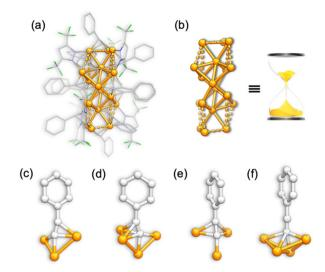
Fig. 3 The crystal structure of  $Cu_{18}$ . (a) The overall structure; (b) metal core and (c), (d), (e) and (f) four types of ligation mode of an alkyne in  $Cu_{18}$ .
