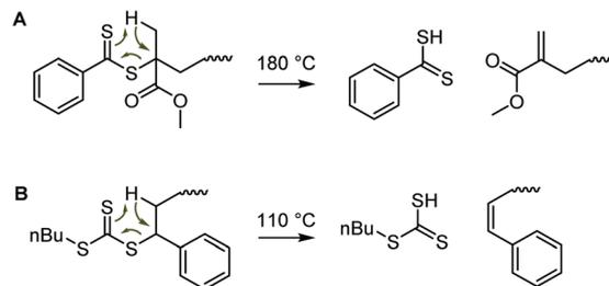
**Scheme 32** (A) Thermal Chugaev eliminations on dithiobenzoate-terminated poly(methyl methacrylate)<sup>184</sup> and (B) trithiocarbonate-terminated polystyrene.<sup>183</sup> Both reactions provide intact polymers with terminal unsaturation. The respective RCSSH products are unstable and degrade further.
