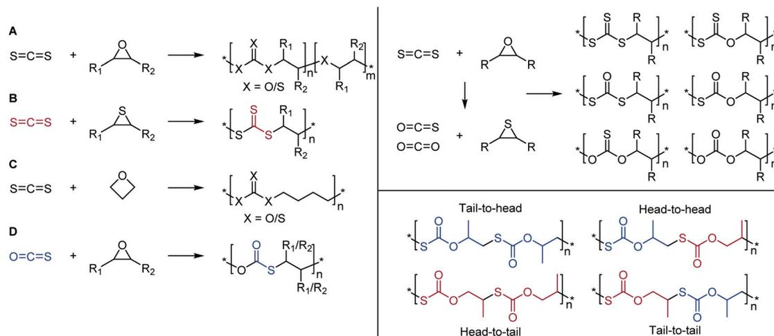
**Scheme 20** Left: Copolymerization reactions of carbon disulfide with (A) epoxides, (B) thiiranes, (C) oxetane, and (D) copolymerization with carbonyl sulfide and epoxides; Right top: O/S scrambling of  $\text{CS}_2$  and epoxides leading to a large range of backbone polymer moieties; Right bottom: copolymerization of  $\text{COS}$  and propylene oxide leading to different polymer microstructures. Adapted from ref. 133 with permission from the American Chemical Society, copyright 2016.
