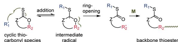
**Scheme 12** Mechanism of thiocarbonyl addition-ring-opening (TARO) radical polymerization.
