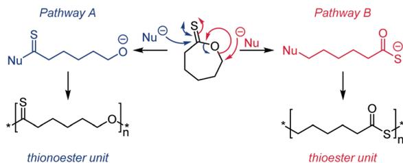
**Scheme 17** The two potential mechanisms for AROP of  $\epsilon$ -thionocapro lactone, **16**. Pathway A: use of a strong nucleophile, such as an organolithium reagent, formed thionoester polymers; Pathway B: use of a poor nucleophile, such as DBU, formed thioester polymers through an S–O isomerisation. Adapted from ref. 100 with permission from the American Chemical Society, copyright 1999.
