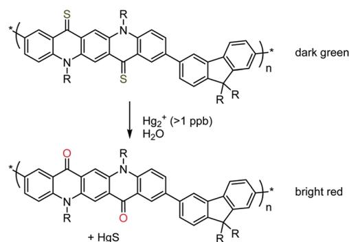
**Scheme 33** Mercury-sensing conjugated polymer that changes colour based on the catalysed dethionation of two thiocarbonyl groups. Reproduced from ref. 187 with permission from the Royal Society of Chemistry, copyright 2014.
