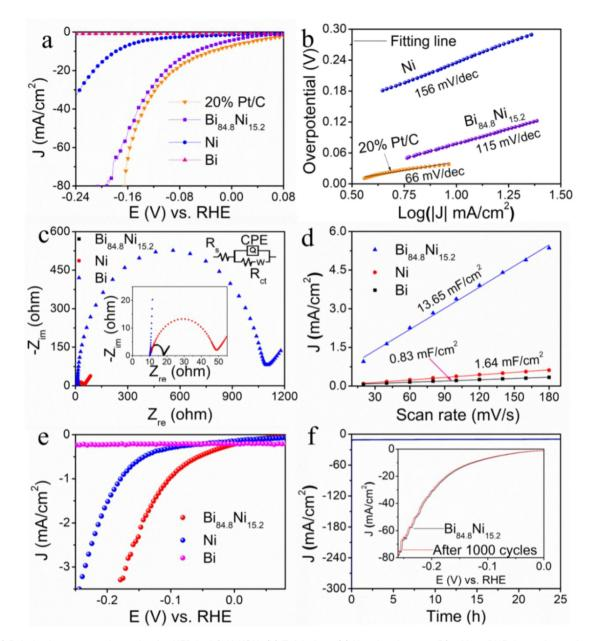
Fig. 2 (a) Polarization curves of samples for HER in 1.0 M KOH; (b) Tafel plots; (c) Nyquist plots at -56 mV vs. RHE. Inset shows the equivalent circuit; (d) capacitive current as a function of scan rate for the samples; (e) specific activity; (f) I-t test for Bi<sub>84.8</sub>Ni<sub>15.2</sub> alloy at -56 mV vs. RHE; inset shows the polarization curves at 5 mV s<sup>-1</sup> before and after 1000 cycles of CV.
