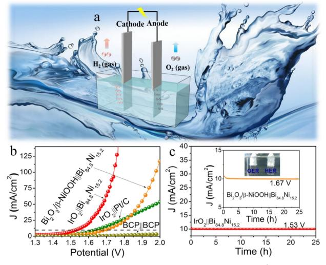
Fig. 5 Overall water splitting performance (a) two-electrode device; (b) polarization curves at a scan rate of 5 mV s<sup>-1</sup>; (c) I-t curves at an invariant cell voltage; Inset: image taken during water splitting.
