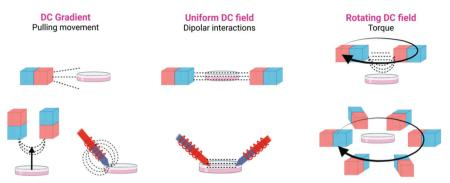
Fig. 2 Different configurations of DC magnetic field applicators commonly used in magnetogenetic experiments, using either permanent magnets or electromagnets. Figure created with BioRender.com.
