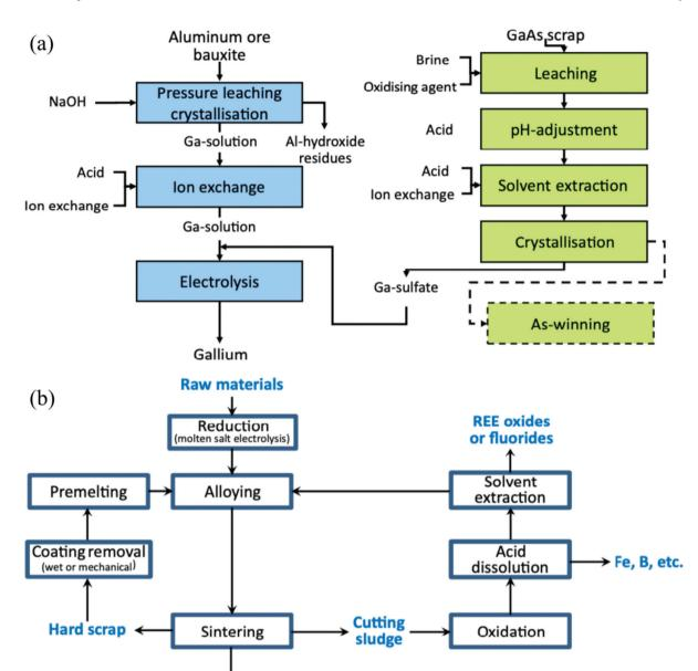
Fig. 4 (a) Process scheme for the recovery of Ga from common feedstocks. (b) Process scheme for the recycling of REEs from permanent magnet waste. Both panels reproduced from ref. 92 with permission from Elsevier, 2014.
