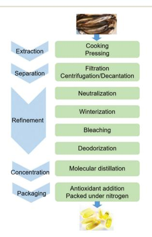
Fig. 2 The conventional procedure of industrial production of marine omega-3 FA supplements.
