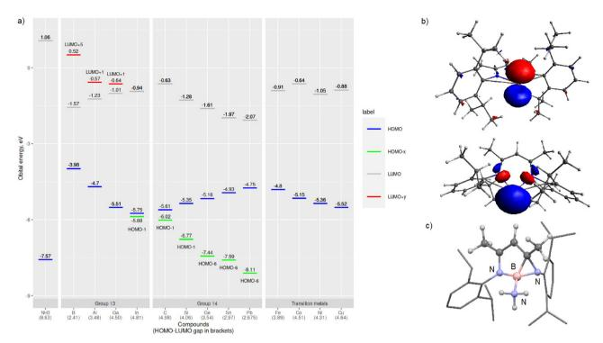
Fig. 2 (a) Calculated HOMO–x and LUMO+y energy levels for the computed LM/L'M species. HOMO–x indicates a lone pair MO and LUMO+y an empty p-orbital associated with the main group element M, (b) LUMO+1 (upper) and HOMO (lower) of LGa (isovalue set at  $\pm 0.05$  a.u.), and (c) structure of the rearranged LB·NH<sub>3</sub>, Dipp-groups are shown as a wireframe format for clarity.
