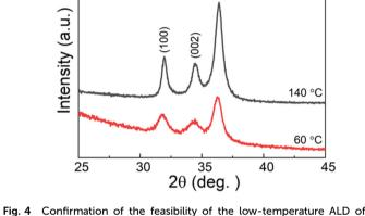
Fig. 4 Confirmation of the feasibility of the low-temperature ALD of ZnO films from  $[Zn(DMP)_2]$  and  $H_2O$  precursors: (a) saturation study of the  $[Zn(DMP)_2]$ : the  $H_2O$  pulse kept constant at 2 s and the  $[Zn(DMP)_2]$  pulse varied; deposition was performed at 60 °C. (b) GIXRD of ZnO deposited on Si(100) at two different temperatures. The total number of cycles was 600 in both cases, the reflections are indexed.
