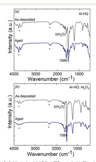
Fig. 3 Stability studies of Al-HQ films: FTIR spectra for (a) a 70 nm thick Al-HQ film immediately after the deposition and aging (two-week) in ambient conditions, and (b) Al-HQ film deposited at 140 °C and capped with 45 nm Al<sub>2</sub>O<sub>3</sub> layer measured immediately after the deposition and after one-week storage in ambient conditions. The bands marked with \* are caused by adsorbed CO2.
