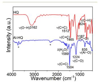
Fig. 2 FTIR spectrum of a 70 nm thick Al-HQ thin film deposited on Si at 140 °C. For comparison the spectrum recorded for the HQ precursor is also shown. The bands marked with \* are caused by adsorbed CO2.
