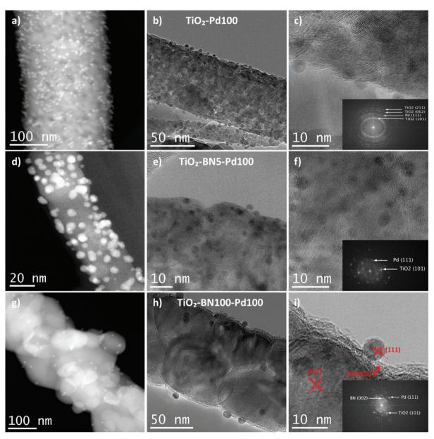
Fig. 4 TEM and HRTEM images of (a-c) TiO<sub>2</sub>-Pd100; (d-f) TiO<sub>2</sub>-BN5-Pd100 and (g-i) TiO<sub>2</sub>-BN100-Pd100.
