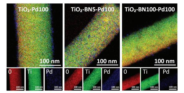
Fig. 5 EDS elemental mapping of TiO<sub>2</sub>-Pd100, TiO<sub>2</sub>-BN5-Pd100 and TiO<sub>2</sub>-BN100-Pd100 nanofibers.
