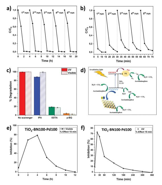
Fig. 11 Recycling test of  $TiO_2$ -BN100-Pd100 under (a) visible and (b) UV irradiation; (c) scavenger plot for determining reactive species in the degradation of ACT by  $TiO_2$ -BN100-Pd100; (d) mechanism of ACT degradation by  $TiO_2$ -BN100-Pd100; inhibition of luminescence of *V. fischeri* marine bacteria during ACT photocatalysis after 15 min exposure between the bacterial strain and the degradation solution under (e) visible and (f) UV irradiation.
