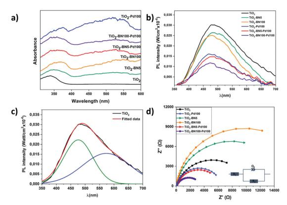
Fig. 8 (a) UV-Vis diffused reflectance of TiO<sub>2</sub> NFs and nanocomposites; (b) photoluminescence of all synthesized NFs; (c) deconvolution of TiO<sub>2</sub> PL spectra; and (d) EIS Nyquist plots of prepared nanofibers.
