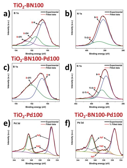
Fig. 7 Deconvoluted XPS spectra of B 1s (a and c), N 1s (b and d) and Pd 3d (e and f) for modified TiO<sub>2</sub> by ALD.
