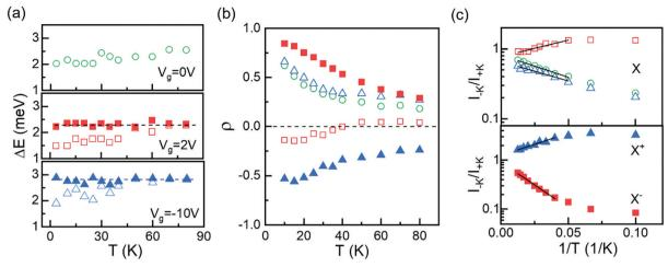
Fig. 4 Temperature dependency of repulsive polarons (open symbols) and attractive polarons (solid symbols) at  $V_{\rm q}=0$  (green),  $V_{\rm q}=2$  V (red), and  $V_q = -10 \text{ V}$  (blue) for (a) polaron energy splitting, (b) valley polarization, and (c) intensity ratio of  $\sigma^+$  and  $\sigma^-$  emission. Spectra were taken with linearly polarized excitation at 1.662 eV. In (c) the solid black lines are fits for extracting thermal activation energy
