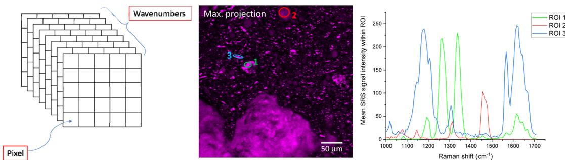
**Fig. 8** Hyperspectral SRS imaging schematic (left); maximum intensity projection of a hyperspectral SRS stack acquired by recording SRS images of the sample with 0.1 nm increments in wavelength of the pump beam (middle); resulting SRS spectra generated from the ROIs indicated (right).
