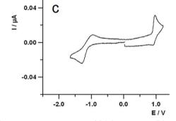
Fig. 4 Cyclic voltammetric curves of (a) 0.6 mM species 3 (three scans at different inversion potential); (b) 0.7 mM compound C<sub>60</sub>-Ph (blue line) and 5 (red line); (c) 0.7 mM species 4 recorded in TBAH/DCM at 298 K. Scan rate =  $1 \text{ V s}^{-1}$ ; working electrode: platinum disk (diameter 125  $\mu$ m); reference electrode: SCE.
