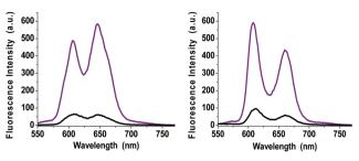
Fig. 6 Steady-state fluorescence spectra of ZnP (purple line) and ZnP-2EDOTV- $C_{60}$  (1, black line) in toluene (left) and benzonitrile (right).  $\lambda_{\rm exc}$  = 426 nm. Concentration 10<sup>-6</sup> M
