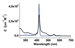
Fig. 4 UV-visible absorption spectra of ZnP-2EDOTV-C<sub>60</sub> (1, black) and **ZnP** (blue) in dichloromethane solution. Concentration:  $10^{-5}$  M.
