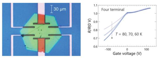
Fig. 9 Microscope image of the thin hexagonal crystal of  $[(S)-1]_9(Mo_6O_{19})_5\cdot(CHBr_3)_2$  attached on the  $SiO_2/Si$  substrate with pre-patterned gold electrodes (left). Gate voltage dependence of normalized resistance of the crystal at selected temperatures of 60 K, 70 K, and 80 K (right).
