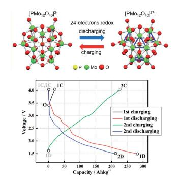
Fig. 5 Structures of POMs  $[PMo_{12}O_{40}]^{3-}$  and  $[PMo_{12}O_{40}]^{27-}$ . Charging and discharging curves of a POM/Li battery. Extracted from ref. 127.
