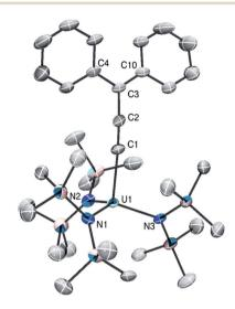
Fig. 2 Solid-state structure of [Li(2.2.2-cryptand)][{(NR<sub>2</sub>)<sub>3</sub>}U(CCCPh<sub>2</sub>)] (3) shown with 50% probability ellipsoids. Hydrogen atoms, [Li(2.2.2-cryptand)], and pentane solvate omitted for clarity.
