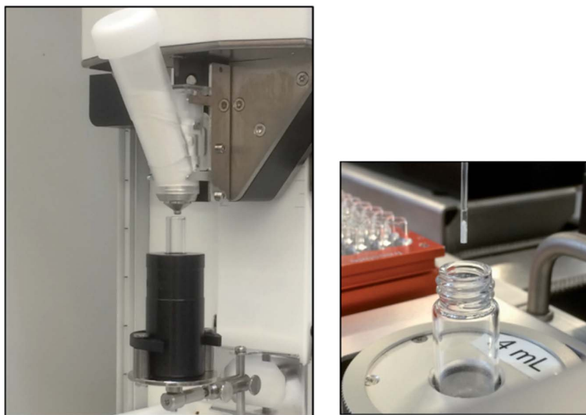
Fig. 3 Axelsemrau Chronect outfitted with a Mettler-Toledo Auto Chem Quantos solid dispense module (left). Chemspeed Technologies GDU-S SWILE with a positive-displacement module (right). Reprinted with permission from ref. 13. Copyright 2020 American Chemical Society.
