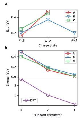
Fig. 5 (a) Addition energies from experimental stability diagrams for devices A–C. (b) The Hubbard parameters for the devices that reproduce these addition energies (upper panel) along with DFT calculations of these values (lower panel).
