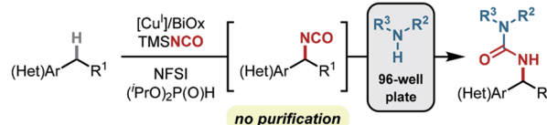
Fig. 1 Copper-catalyzed benzylic C(sp 3 )–H isocyanation/amine coupling. (A) Drug candidates embedding benzylic urea. (B) Two possible one-pot synthetic approaches toward ureas from benzylic C–H substrates. (C) Strategy for high-throughput synthesis of ureas. NFSI, N -fluorobenzenesulfonimide; BiOx, 2,2′-bis(oxazoline); TMSNCO, (trimethylsilyl)isocyanate.
