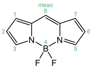
Fig. 1 Structure of the BODIPY core and IUPAC numeration.
