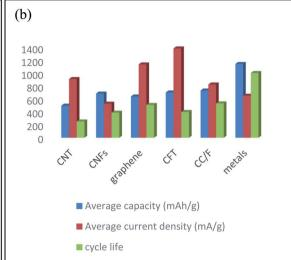
Fig. 10 (a) Average initial capacities at the average current densities, and (b) average capacities, average current densities, and average cycle life of all types of electrodes (these data also collected from the same sources as reported in Fig. 8).
