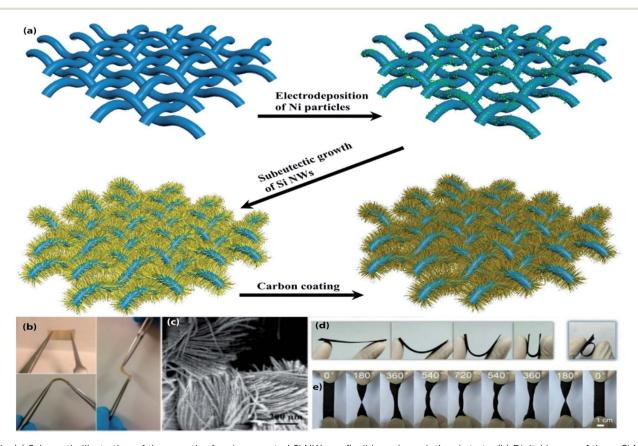
Fig. 4 (a) Schematic Illustration of the growth of carbon-coated Si NWs on flexible carbon cloth substrate. (b) Digital image of the c-Si NWs/carbon cloth electrode, (c) representative SEM image of the c-Si NWs/carbon cloth electrode. (a–d) Reprinted from ref. 111. (d and e) Photographs of the flexible CF@SnO<sub>2</sub>-NS@AC electrode during the folding, the rolling, and twisting tests. (d and e) Reproduce with permission, <sup>124</sup> copyright 2018, Elsevier.
