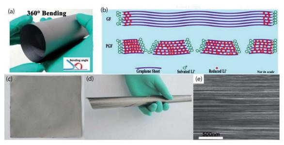
Fig. 6 (a) Digital image of porous graphite film (PGF) being bent 360°, (b) a simple schematic illustration of the lithium intercalation into flexible graphite film and flexible PGF. Reprinted from ref. 151. (c) The image as prepared pyrolytic graphite film (PyGF), (d) rolled image of PyGF, (e) crosssectional SEM image of PyGF. (c-e) Reprinted from ref. 149.
