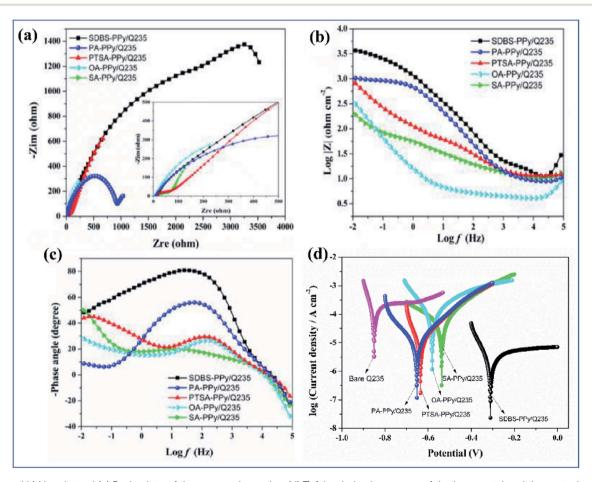
Fig. 13 (a and b) Nyquist and (c) Bode plots of the prepared samples. (d) Tafel polarization curves of the bare metal and the coated polypyrrole films (DOI: 10.20964/2020.03.49, open source ESG).
