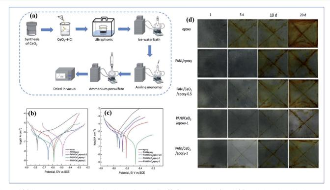
Fig. 12 (a) Schematic representation of synthesis route for polyaniline/ $CeO_2$  nanoparticles. (b and c) Potentiodynamic polarization curve of control epoxy coating and conducting polymer composite pigmented coating after 1 and 15 days, respectively. (d) Salt spray test results after 20 days for epoxy coating, PANI/epoxy coating, PANI/ $CeO_2$ /epoxy-0.5 coating, PANI/ $CeO_2$ /epoxy-1 coating, and PANI/ $CeO_2$ /epoxy-2 coating (reprinted with permission, 156 copyright 2019 Elsevier).
