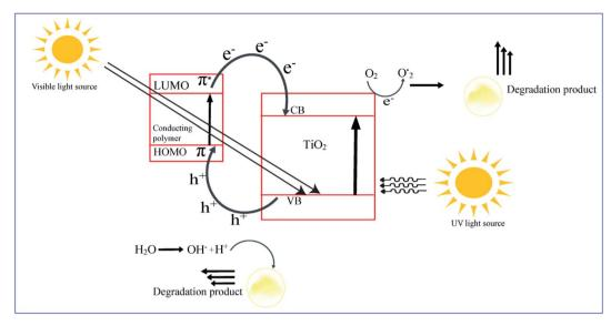
Fig. 15 Photocatalytic mechanism in conducting polymer composites.
