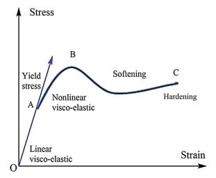
Fig. 8 Typical stress-strain curve of polymeric materials.
