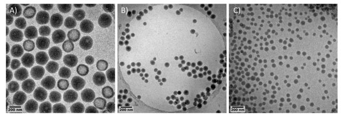
Fig. 1 Cryo-TEM images of PVDF particles prepared with (A) PEG-OH (L01), (B) PEG-SH (L04) and (C) PEG-X (L03).
