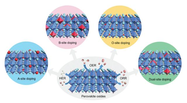
Fig. 1 Schematic illustration of the A-site, B-site, O-site and dual-site heteroatom doping of ABO<sub>3</sub>-type perovskite oxides for efficient electrocatalytic reactions including the HER, OER and ORR.
