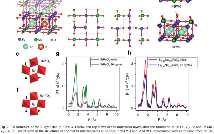
Vo-Fe. (d) Lateral view of the structures of the \*OOH intermediates at Fe sites in KSFMO and in SFMO. Reproduced with permission from ref. 48. Copyright 2017, Royal Society of Chemistry. Schematic representation of octahedral distortion in (e) SrRuO3 and (f) Sr0.9Na0.1RuO3. Fourier transform from Ru K-edge EXAFS signals of (g) SrRuO3 and (h) Sr0.9Na0.1RuO3 before and after OER cycles. Reproduced with permission from ref. 49. Copyright 2019, Nature Publishing Group.
