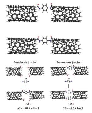
Fig. 12 Schematic of a PPD (p-phenylenediamine)-linked molecular junction and reactions of formation for linear junctions with one and two bringing molecules. Reprinted with permission from Zhu et al., J. Am. Chem. Soc., 2016, 9, 2905. Copyright 2016 American Chemical Society.
