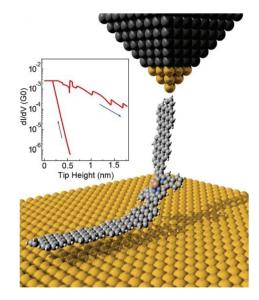
Fig. 11 Illustration of the target experimental geometry. The inset shows a typical conductance-distance plot simultaneously recorded during tip approach and retraction. Reprinted with permission from Li et al., Nano Lett., 2019, 19, 3288. Copyright 2019 American Chemical Society.
