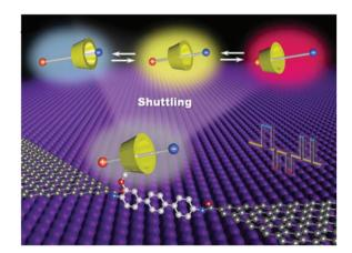
Schematic of the device structure of GMG-SMJs formed by individual molecular shuttles. Reprinted with permission from Zhou et al., Small Methods, 2019, 3, 1900464. Copyright 2019 Wiley-VCH Verlag
