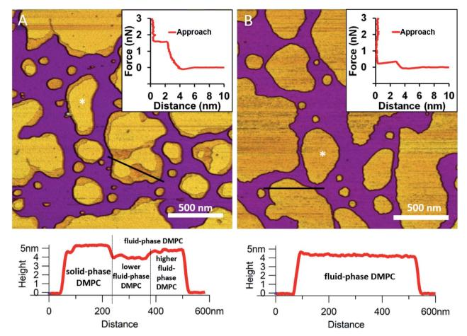
Fig. 1 Height-contrast AFM images of DMPC SLBs: DMPC SLBs imaged at  $20\,^{\circ}$ C (A). DMPC SLB heated to  $30\,^{\circ}$ C (B). Insets: force—distance curves recorded while rupturing DMPC at the locations marked by the white star on each image. Lower panels show the height-distance functions along the black lines indicated on the images.
