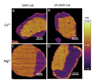
Fig. 4 Height-contrast AFM image of DMPC SLB (A and C); LPS-DMPC SLB (B and D); on mica at 20  $^{\circ}$ C in the presence of 10 mM Ca<sup>2+</sup> (A and B); in the presence of 10 mM Mg<sup>2+</sup> (C and D) respectively. Orange and purple indicate solid and fluid states, respectively.
