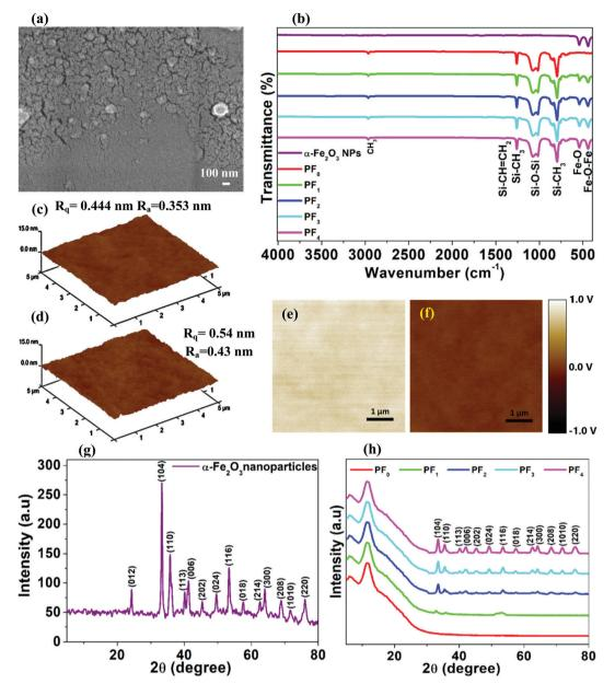
Fig. 2 (a) FESEM view of the PF<sub>2</sub> film and (b) FTIR spectra of  $\alpha$ -Fe<sub>2</sub>O<sub>3</sub> NPs, PDMS, and PDMS@ $\alpha$ -Fe<sub>2</sub>O<sub>3</sub> NP composites; AFM images (three-dimensional) of the (c) PDMS film and (d) PF<sub>2</sub> film; KPFM images of (e) PDMS film and (f) PF<sub>2</sub> film. XRD plots of (g) α-Fe<sub>2</sub>O<sub>3</sub> nanoparticles and (h) PDMS@α-Fe<sub>2</sub>O<sub>3</sub> NP composites
