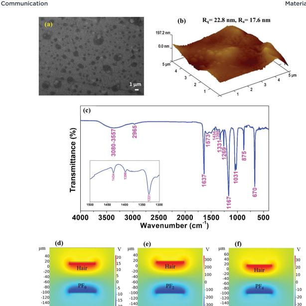
Fig. 3 (a) FESEM view of the human hair-based film. (b) AFM image (three-dimensional) of the human hair-based film. (c) FTIR spectra of the human hairbased film with an expanded spectrum view of a certain region (1300-1500 cm<sup>-1</sup>) in the inset. COMSOL simulation results of the TENGs comprising the human hair based film and (d) PF<sub>0</sub>, (e) PF<sub>2</sub>, and (f) PF<sub>4</sub> film.
