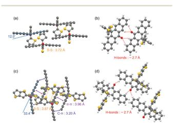
Fig. 1 Crystal structure of 1: (a) the dihedral angle of the pentacenone unit and sulfur-sulfur interactions (hydrogens have been removed to clarify the view); (b) hydrogen bonds. Crystal structure of 2 (the two isomeric thienothiophene rings are in a disordered structure): (c) the dihedral angle of the pentacenone unit, sulfur-sulfur interactions and aromatic interactions (hydrogens have been removed to clarify the view); (d) hydrogen bonds.
