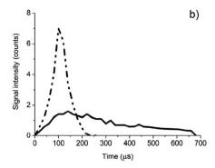
Fig. 7 A comparison of the high time resolution signal profiles for 30 nm diameter spherical gold NPs (panel a) and for 2.63 aspect ratio gold nanorods (panel b). In each panel, the two extreme time profiles (with the shortest (dashed dotted line) and longest (solid line) durations observed) as averages for 40-50 particles are shown. 313
