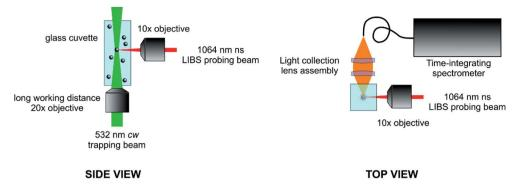
Scheme of an experimental arrangement for LIBS analysis of optical trapped single nanoparticles.
