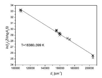
Fig. 1 Saha–Boltzmann plot constructed from the emission spectrum of a Cu/Ar spark discharge plasma measured  $\it ca.$  1  $\mu s$  after the onset of the gas breakdown (based on the authors' own data).
