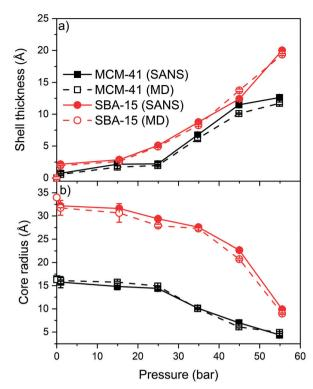
Fig. 7 The thickness of the adsorbed CO<sub>2</sub> layer determined from the small-angle neutron scattering measurements and molecular dynamics simulations (a) and the corresponding core radius (b) as a function of the applied pressure are shown. The error bars of the SANS and MD data represent standard deviations based on fittings and simulations performed in triplicates.
