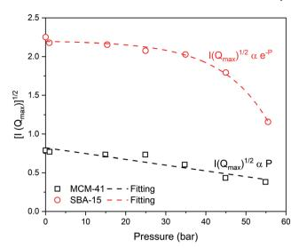
Fig. 4 The amplitudes of the SANS intensity  $[I(Q_{\rm max})^{1/2}]$  at the maximum of the first-order peak as a function of the applied pressure in MCM-41 and SBA-15 pores are shown. The pressures at which the intensity reaches zero average contrast in MCM-41 and SBA-15 are about 110 bar and 72 bar, respectively.
