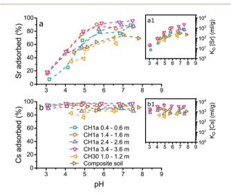
Fig. 2 Graphical representation of the results from the aqueous analyses from the adsorption experiments to the composite clayey soil and the LFLS core samples (initial concentrations of 20 Bg ml<sup>-1</sup> Sr-85 and Cs-137) with the % of Sr (a) or Cs (b) adsorbed plotted against pH, and the respective  $K_D$  values (a1 and b1). The legend represents the location<sup>46</sup> and depth of the LFLS core samples used in the adsorption experiments.
