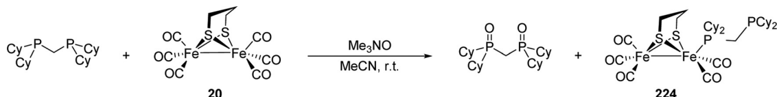
Fig. 66 Reaction of dcmp with complex 20 in the presence of \text{Me}_3\text{NO} .
