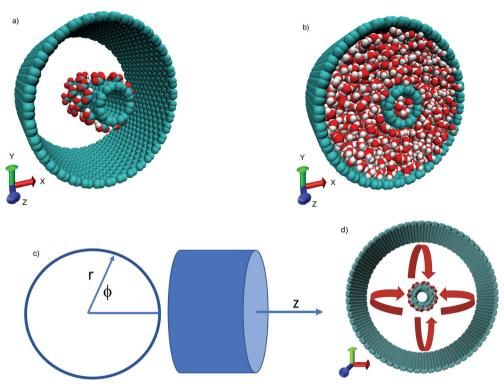
Fig. 8 (a) Concentric carbon nanotubes, with inner tube functionalised with carboxyl groups. (b) System filled with water molecules. (c) Geometry, where r is the radial coordinate from the common centre of the nanotube system,  $\phi$  is the azimuthal angle and z defines the tube axis. (d) Electric field (red) direction of rotation within the concentric nanotube system. Reprinted (adapted) with permission from Ostler et al. 66 Copyright 2019 American Chemical Society.
