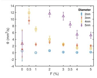
Fig. 7 Net volume flow rate  $\Phi$ , defined as the integrated time averaged velocity over the cross-sectional area of the CNT, as a function of nanotube diameter and percentage functionalisation. Electric field frequency and amplitude are as in Fig. 5. Reprinted (adapted) with permission from Ostler  $et~al.^{64}$  Copyright 2017 American Chemical Society.
