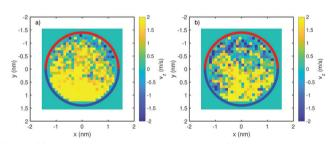
Fig. 5 (a) Plot of water streaming velocity for 2% functionalisation for external electric field frequency of 20 GHz and amplitude 0.032 V Å $^{-1}$ . (b) As for (a) but with 5% functionalisation. Reprinted (adapted) with permission from Ostler *et al.* $^{64}$  Copyright 2017 American Chemical Society.
