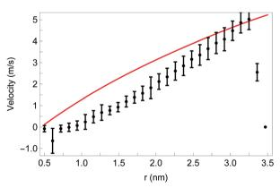
**Fig. 11** Comparison of numerical solution of eqn (49) and (50) (red curve) with NEMD streaming velocity (black points) for a concentric system of 3 nm tube gap and 5% functitonalisation. The external electric field frequency and amplitude were 20 GHz and 0.032 V Å $^{-1}$ , respectively. Reprinted (adapted) with permission from Ostler *et al.* <sup>66</sup> Copyright 2019 American Chemical Society.
