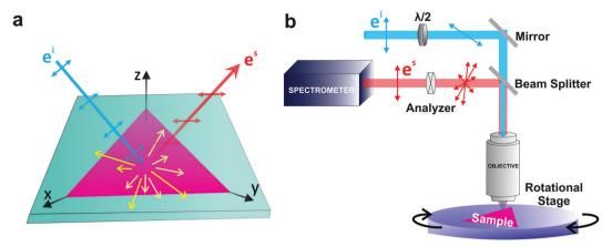
Fig. 1 Schematic of the Raman experiment setup. (a) Schematic of the light-matter interaction giving rise to the Raman scattering process. (b) Schematic of the experimental setup for a polarized Raman measurement.
