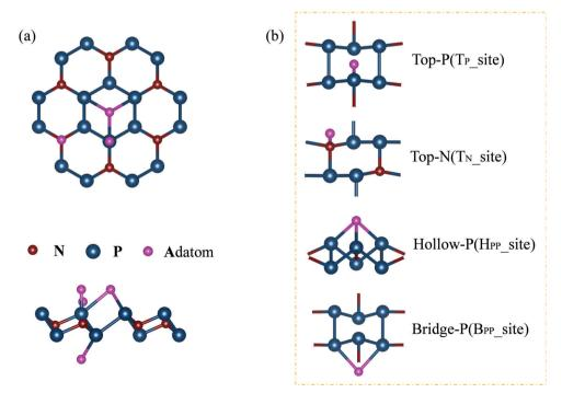
Fig. 3 (a) A schematic illustration of top and side views of the embedded single atom, and (b) adsorption sites of the atoms on monolayer N<sub>2</sub>P<sub>6</sub> as presented in Table 1.
