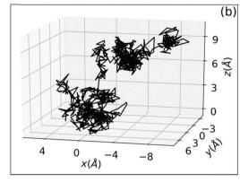
Fig. 6 (a) Correlation length of different species in maline, reline, glyceline and ethaline calculated from eqn (5) using the diffusion constant obtained from PFG-NMR (adapted from ref. 74). (b) MD simulation trajectory of acetamide molecules in DES (acetamide + lithium perchlorate, 78: 22), showing both long-range jumps and the localised diffusion within the cages (adapted from ref. 20).
