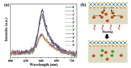
Fig. 4 (a) Reversible modulation of PL intensity for 5 cycles by laser irradiation and thermal annealing. (0) PL spectra of monolayer MoS<sub>2</sub> on P<sup>+</sup> Fe:LiNbO<sub>3</sub> before laser irradiation. (1-5) PL spectra after laser irradiation and (1'-5') restored PL spectra after thermal annealing. (b) Schematic illustration of erasing the charge redistribution in P<sup>+</sup> Fe:LiNbO<sub>3</sub> via thermal annealing.
