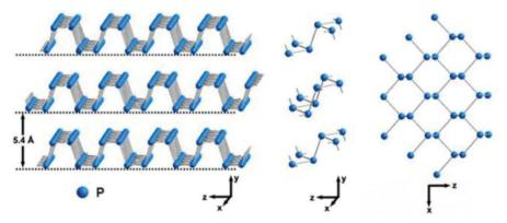
Fig. 9 Crystal structures of BP. Reproduced from ref. 73 with permission from American Chemical Society
