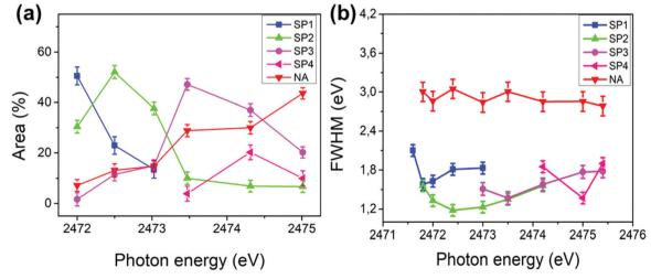
Fig. 5 Area % (a) and full width at half maximum (FWHM) (b) plotted against the incident photon energy of the decay channels (SP1, SP2, SP3, SP4 and NA) in the S K- $L_{2,3}L_{2,3}$  RAS spectra of the PFO-DBT/SiO<sub>2</sub> thin film. The error bar of 3% is also represented.
