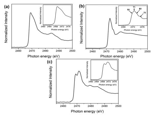
Fig. 2 Sulfur K-edge NEXAFS thin-film spectra of (a) exfoliated franckeite/SiO<sub>2</sub>, (b) PFO-DBT/SiO<sub>2</sub>, and (c) PFO-DBT/Fr.
