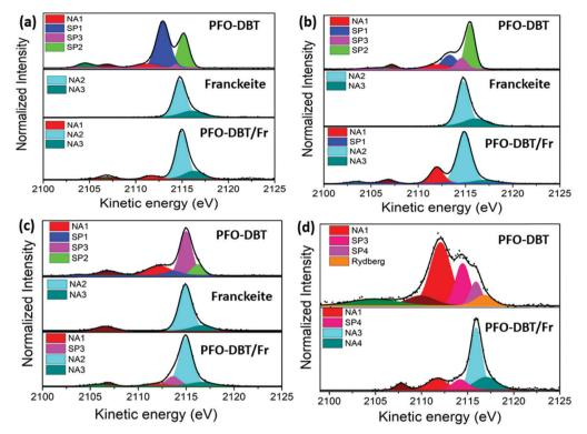
Fig. 4 S K-L<sub>2.3</sub>L<sub>2.3</sub> RAS spectra of PFO-DBT, exfoliated franckeite and PFO-DBT/Fr thin films collected at the photon energies of (a) 2471.8 eV (B1), (b) 2472.5 eV (T1), (c) 2473.5 eV (B2), and (d) 2474.5 eV (T2).
