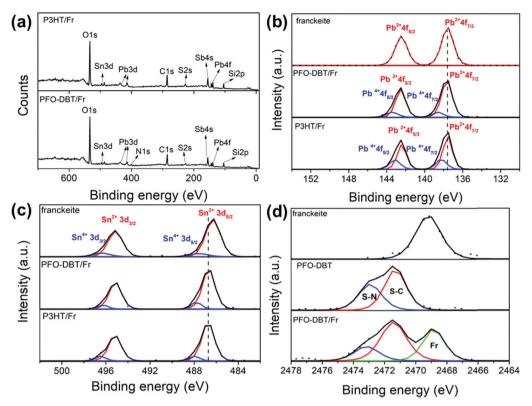
Fig. 1 (a) XPS survey spectra of the PFO-DBT/Fr and P3HT/Fr heterojunctions. (b) and (c) Pb4f and Sn3d high-resolution XPS spectra of exfoliated franckeite and the PFO-DBT/Fr and P3HT/Fr heterojunctions, respectively. (d) S1s high-resolution XPS spectra of exfoliated franckeite and the PFO-DBT/ SiO<sub>2</sub> and PFO-DBT/Fr thin films
