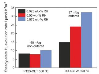
Fig. 23 Comparison of steady-state H<sub>2</sub> evolution rates for disordered and ordered mesoporous CsTaWO<sub>6</sub> with different amounts of Rh co-catalyst. Adapted from ref. 256 with permission.
