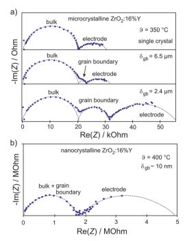
Fig. 6 (a) Impedance spectra for single-crystal and microcrystalline YSZ. The grain boundaries of the microcrystalline sample lead to the appearance of an additional semicircle. (b) Reducing the grain size to the nanometer level results in merging of semicircles representing the bulk and grain boundary transport processes. Adapted from ref. 77 with permission.
