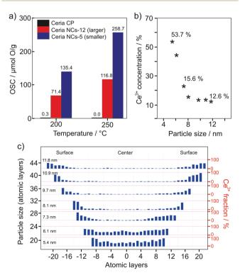
Fig. 18 (a) Comparison of the oxygen-storage capacity of CeO<sub>2</sub> nanoparticles of different size and commercially available nanopowder. (b) Ce<sup>3+</sup> content as function of the particle size and (c) valence-state distribution. Adapted from ref. 226 with permission
