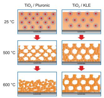
Fig. 2 The effect of annealing temperature on the pore structure of Pluronic- and KLE-templated TiO<sub>2</sub> thin films. Adapted from ref. 54 with permission
