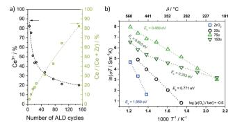
Fig. 30 (a)  $Ce^{3+}$  content of ceria deposited onto mesoporous  $ZrO_2$  thin films as function of the ALD cycle number. The Ce<sup>3+</sup> content decreases with increasing coating thickness. (b) Temperature-dependence of total conductivity for mesoporous ZrO2 and CeO2-ZrO2 composite thin films (25, 75 and 150 ALD cycles). Adapted from ref. 318 with permission.
