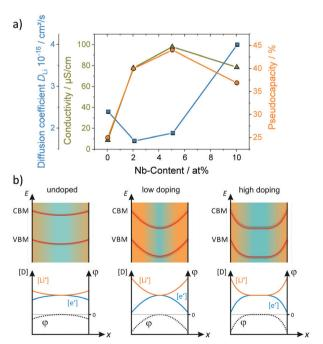
Fig. 16 (a) Electrical conductivity and pseudocapacitive charge storage of mesoporous TiO2 versus the Nb doping level. (b) Schematic illustration of the surface band bending and the corresponding defect concentration for different doping situations. Adapted from ref. 156 with permission.
