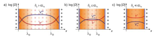
Fig. 7 Defect concentration for different grain sizes (schematically shown for  $CeO_2$ ). (a) The space-charge region affects the defect concentration near the interface in microcrystalline material. (b) For grain sizes smaller than four times the Debye length, the space-charge region starts to overlap and (c) finally completely dominates the defect concentration of the whole grain. Adapted from ref. 78 with permission.
