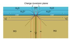
Fig. 12 Schematic illustration of the resistive behavior of a grain boundary with adsorbed water molecules on the surface of an oxide ceramic (MO). Because of the positive core, hydroxide ions accumulate at the grain boundary, impeding the transport of hydronium ions in the physisorbed water layer. Reprinted from ref. 136 with permission.
