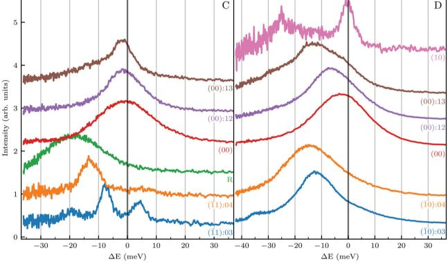
Fig. 1 (Top) Angular diffraction measurement of CH<sub>4</sub> with incident energy of 81 meV along the two main high-symmetry directions of the Ir(111) unit cell. Labels indicate the locations of selected RID peaks, whereby their colors correspond to the TOF measurements shown in the lower panels. (Bottom) TOF measurements in energy exchange scale under the same experimental conditions at selected scattering angles indicated by labels of the same color in panels A and B
