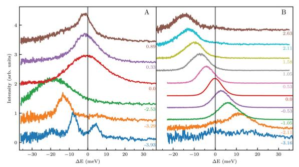
Fig. 4 Comparison of TOF measurements of CH<sub>4</sub> (A) and Ne (B) scattered from the Ir(111) surface ( $T_S = 100$  K) along  $\overline{TK}$  with incident beam energies 81 meV and 69 meV, respectively. The labels indicate the value of the elastic momentum exchange parallel to the surface,  $\Delta K$ , in Å<sup>-1</sup>.
