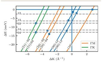
Fig. 2 Maximum energy loss values from the TOF spectra plotted on their corresponding scan curves and compared to the rotational transition energies of CH<sub>4</sub> (gray dashed lines). Scan curve labels indicate the corresponding RID peak from Fig. 1A and B. Scan curves are plotted in orange, green and blue if they correspond to  $\overline{\Gamma M}$ ,  $\overline{\Gamma K}$  or both directions, respectively.
