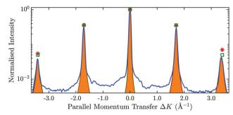
Fig. 7 The blue line shows the scattered intensity versus the parallel momentum transfer along the  $\overline{\Gamma M}$  azimuth of Sb<sub>2</sub>Te<sub>7</sub>(111). The orange areas show the fitted measured intensities based on a Voigt-profile, resulting in a value displayed as red stars. The green squares correspond to the calculated values based on elastic quantum-mechanical scattering calculations
