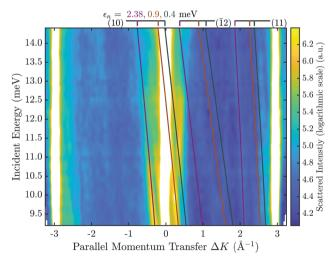
Fig. 6 Contour plot of the scattered He intensity in dependence of momentum transfer and incident energy along the  $\overline{\Gamma K}$  azimuth, for the Sb<sub>2</sub>Te<sub>3</sub>(111) sample at 113 K. The solid lines are the positions of the SAR features according to the free atom model with the different colours denoting the bound state energies  $\varepsilon_{1,2,3}$ . The Miller indices of the interacting G-vectors are given in brackets
