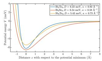
Fig. 9 Comparison of the laterally averaged potentials  $V_0(z)$  for the binary TIs based on the determined corrugated Morse potentials in Table 1.
