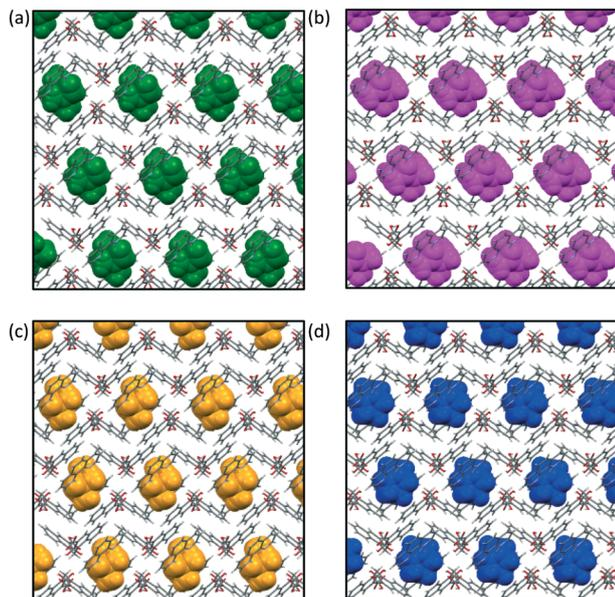
Fig. 1 The isostructural solvates of **1** (1,10-phenanthronium pamoate). (a) **1-DMF**, (b) **1-DMA**, (c) **1-DMSO** and (d) **1-THF**. The host ions are shown in stick representation, whilst the guest molecules are shown in spacefill representation with each guest in a different colour.
