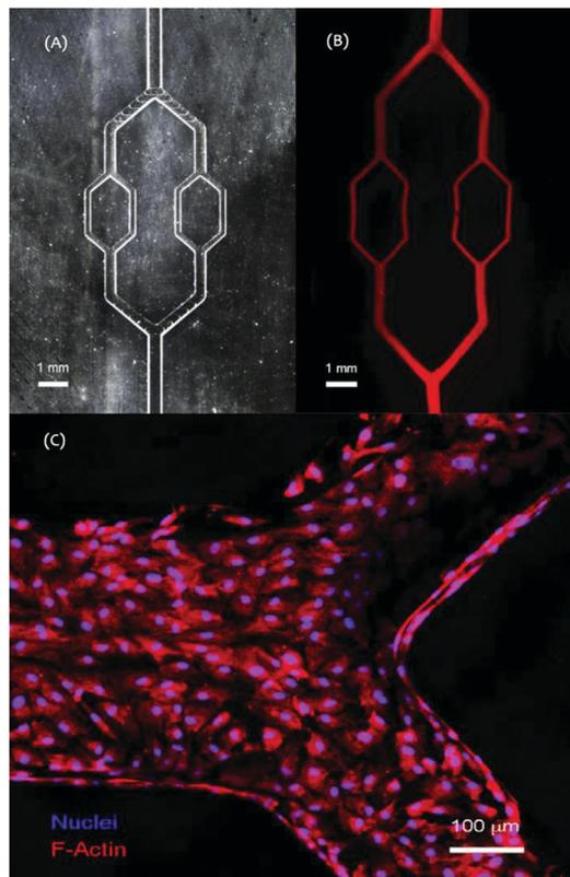
**Fig. 5** Using a sacrificial mold to make microfluidic channels in hydrogel. (A) Image of the sacrificial mold made from PVA using an etched glass pattern. (B) After the PVA mold was removed from the cured hydrogel around it, hollow channels were formed. The image shows fluorescent microspheres flowing through the channels. (C) An immunofluorescent image of HUVECs seeded on the inside of the channels as blood vessel mimics. Reprinted from Tocchio *et al.* (2015) with permission.
