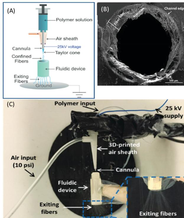
**Fig. 12** Using dynamic focusing to confine microfibers into a fluidic device. (A) The electrospinning setup with air sheath to focus the fibers into a fluidic channel. (B) An SEM image of the cross-section of a device showing a layer of electrospun fibers was deposited on the inside of the channel. (C) The real picture of the setup. Fibers exiting from the other end of the fluidic device (inset) suggest successful fiber focusing. Reprinted from Chen *et al.* (2016) with permission.
