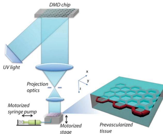
**Fig. 6** Schematic of bottom-up 3D printing with optical curing. A thin layer of prepolymer is loaded onto the motorized stage and the optics are used to select regions for crosslinking. Unpolymerized material is washed off, the stage lowered, and additional layers are loaded on top and crosslinked to build a 3D device. Reprinted from Zhu *et al.* (2017) with permission.
