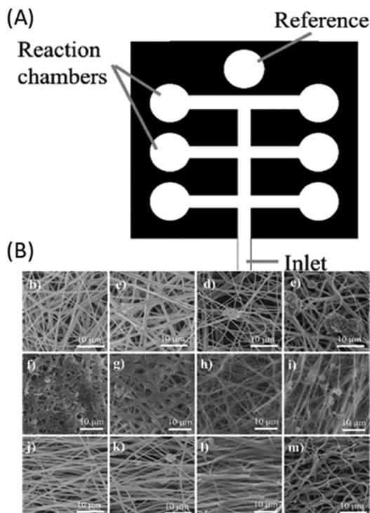
**Fig. 11** (A) The layout of the lateral-flow device created by Pimentel *et al.* On a piece of electrospun fibers, certain areas are blocked (black) with the rest defined as channels and chambers, where liquid can be delivered via capillary actions. (B) Electrospun fibers with various microstructures were tested for cell culture. Reprinted from Pimentel *et al.* (2020) with permission.
