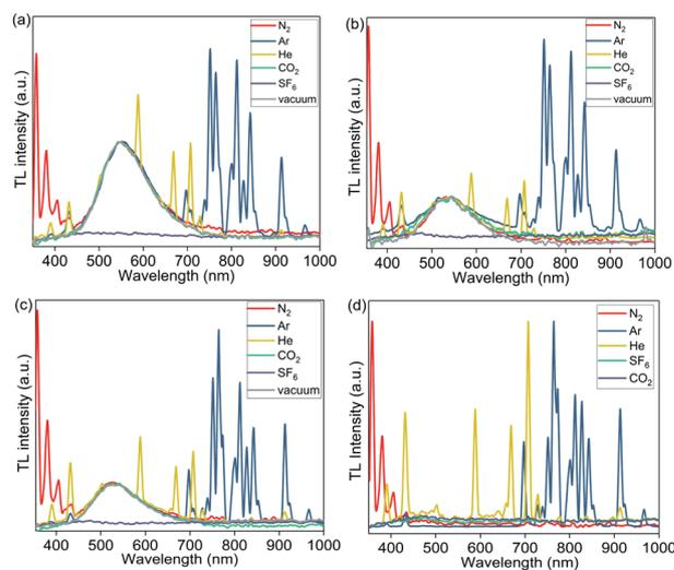
Fig. 6 TL spectra of PMMA films containing 1 wt% of complexes (a) **1**; (b) **2**; (c) **3a**; and (d) PMMA (without Cu complex) recorded under 1 atm of N<sub>2</sub>, Ar, He, CO<sub>2</sub>, SF<sub>6</sub>, and vacuum (0.5 Torr).
